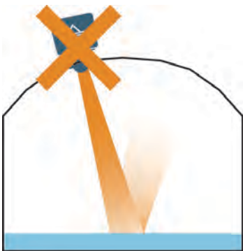
Avoid Mounting at an Angle
