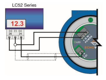
**Note:** LC52 shipped from factory with jumper in JWA mode. Jumper must be switched to JWB mode for operation with the EchoWave®.
