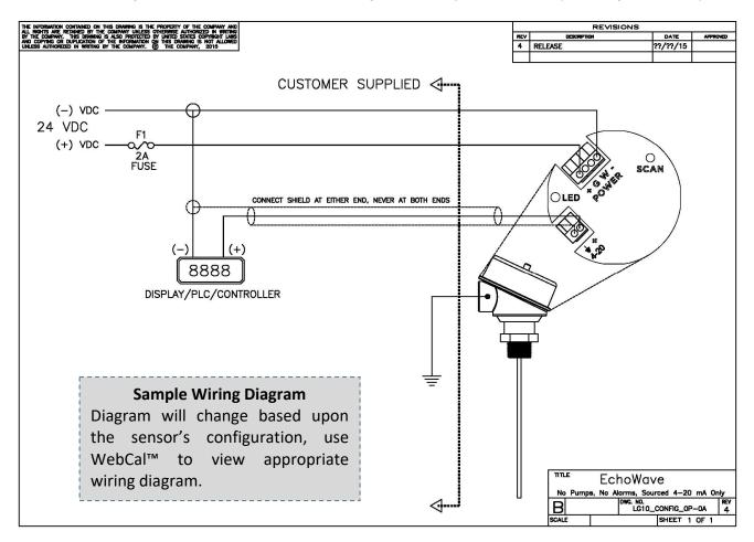
The cabling should be shielded and twisted to minimize EMI interference. Its shield should be connected at either end and **never connected at both ends**. Typically 18 to 24 gauge wire is used in this application.
