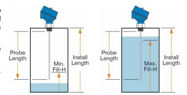
**Note:** Never allow the liquid to rise into the top dead band of the sensor (within 4" from the top of the threads.
