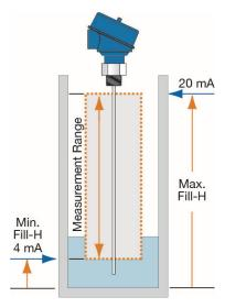
**Distance (Height of Liquid):** When the EchoWave® is configured to read the distance (height of the liquid), the default for the sensor Empty will be at the bottom of the measurement range (end of the probe minus the bottom dead band). This is where 4mA will be set. The default for sensor Full will be at the top of the measurement range (Top Dead Band), where 20mA will be set. The 20mA can be set by the Maximum Fill-Height.
