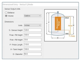
**Tank Height:** Distance from the bottom of the tank to the top of the straight side wall.
