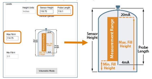
**Note:** In the Distance Mode, the 4mA location will always be 2" from the end of the probe. The Min-Fill-H value will always indicate the distance the 4mA location is above the bottom of the tank.
