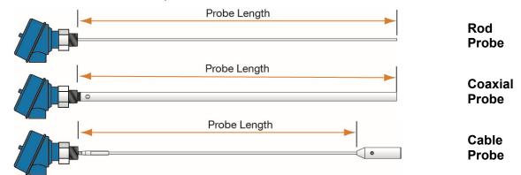
Note: Sensor Height and Probe Length have different reference points for measurement.
