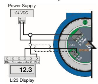
**Note:** 4-20 mA signal wire requires shielding (power supply wires may use the same shielding as the signal wire). Shield wire can be connected at either end. **Never** connect shield wire at **both ends**. EchoWave is a 3-wire transmitter and should never be wired as a 2-wire loop device.
