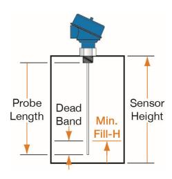
**Note:** Because of the bottom dead band, the Minimum Fill-Height can never be at the end of the probe.
