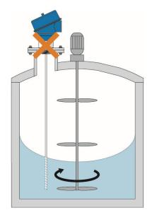
agitator or mixer swirls. In applications with very strong fluid movements which can also cause excessive lateral force on the probe, it is recommended to anchor the probe. The anchoring fixtures are end user supplied.
