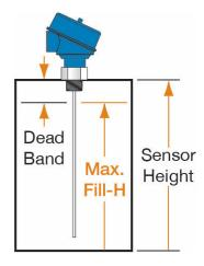
**Note:** Because of the top dead band, the Maximum Fill-Height can never be at the bottom of the threads.
