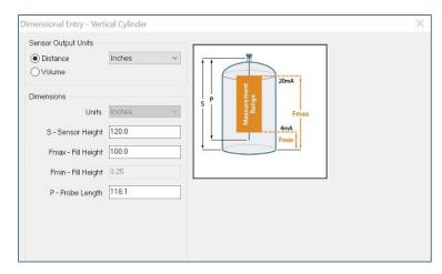
**Probe Length:** Distance of the probe from the bottom of the threads (feed through) to the end of the probe.
