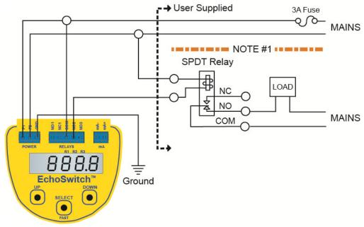
**Note:** – Isolate power to instrument from power to load (pumps, etc.) as much as possible by running power to the sensor directly from main power source.
