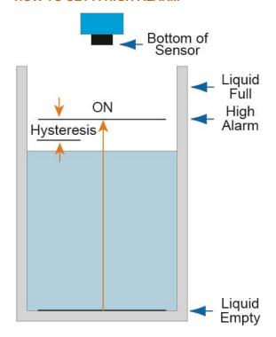
Before starting, measure the distance from the bottom of the tank to the High Alarm position (ON) in the tank.
