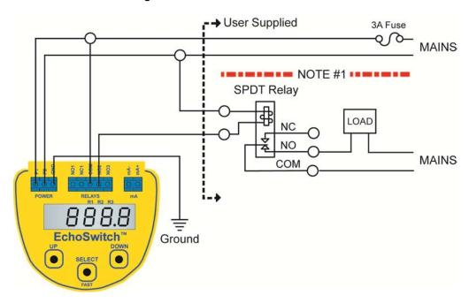
• **Note #1** – Isolate power to instrument from power to load (pumps, etc.) as much as possible by running power to the sensor directly from main power source.
