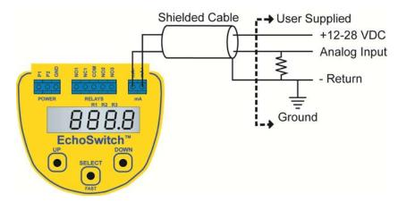
The cabling should be a shielded twisted pair to minimize EMI interference. Typically 20 to 24 gauge wire is used in this application. The analog output of the EchoSwitch® is isolated from the AC power via optocoupler isolation.
