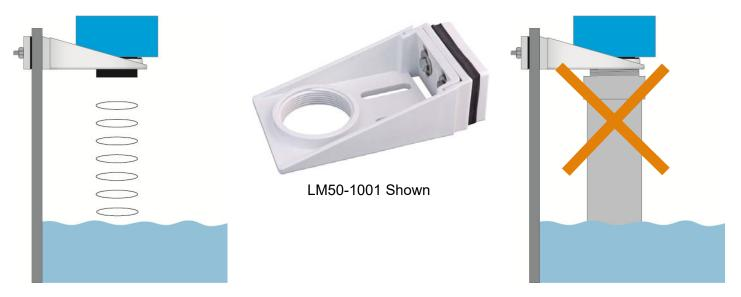
**Note:** The Side Mount Bracket (LM50 series) is not designed for use with stand pipes or as a method to secure stand pipes. There are too few threads to properly hold the sensor and the stand pipe.
