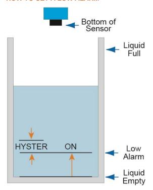
Before starting, measure the distance from the bottom of the tank to the Low Alarm position (ON) in the tank.
