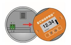
**Note:** There is an internal configuration difference between displays used by the EchoPro® sensors (LR11, LR16, LR21 and LR26 series) versus the display used with the LR98 series. A colored dot on the back marks displays to be used only with the LR98 series. Never swap displays between the LR98 series and other EchoPro® sensors.
