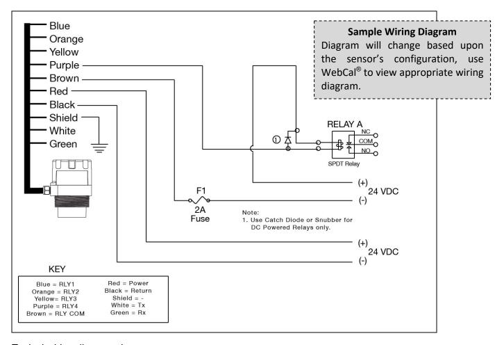
Typical wiring diagram shown.
