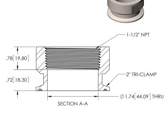
Flowline Part Numbers LM52-1880 = adapter, 1 1/2" NPT to 2" tri-clamp, 316L
