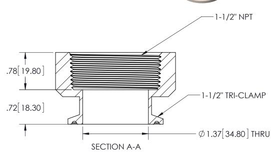
Flowline Part Numbers LM53-1S80 = adapter, 1 1/2" NPT to 1 1/2" tri-clamp, 316L
