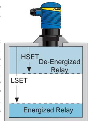
**SAF1/SAF2:** The 10A relay inside the LU30 can be used in a fail-safe design of your system. When [SAF1] is set, the relay will de-energize when the acoustic return signal is LOST. When [SAF2] is set, the relay will energize when the acoustic return signal is LOST. Response times will vary according to the setting of the LU30 ([FAST] or [SLOW] modes).
