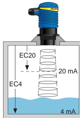
**EC4:** The 4 mA setting for the LU30. The EC4 is the distance from the bottom of the LU30 to the 4 mA set point. This setting is measured in either inches or centimeters on the display. The EC4 setting is typically greater than the EC20 setting.
