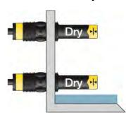
In this state, the relay will never switch, regardless if this is an Auto Fill or Auto Empty application. In this state, the relay will typically energize for an Auto Empty application and will typically deenergize for an Auto Fill application. In this state, the relay will typically energize for an Auto Fill application and will typically de-energize for an Auto Empty application.
