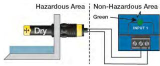
In this state, the relay can be energized with Invert in the OFF setting or can be de-energized with Invert in the ON setting. In this state, the relay can be energized with Invert in the ON setting or can be de-energized with Invert in the OFF setting.
