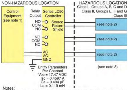
1. Control equipment connected to series LC90 controller must not use or
