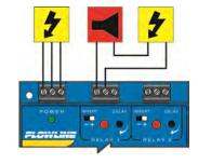
**Note:** The sensor is normally dry. In this condition, we want the relay to be energized so the alarm does not sound: i.e., the Red relay LED should be on whenever the Input LED is Amber. So we turn Invert On. If liquid comes into contact with the switch, the switch activates, the relay de-energizes, and the alarm sounds.
