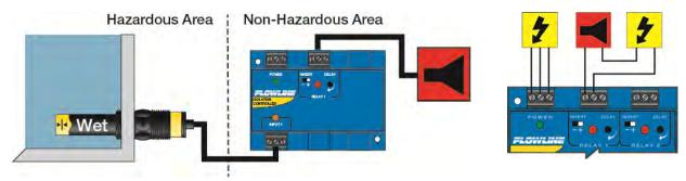
To do this, connect the hot lead of the alarm to the NC side of the relay terminal of the controller. If power is lost, the relay will be de-energized, and the alarm will sound (if there is still power to the alarm circuit itself).
