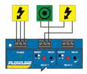
**Note:** In this application, the relay to the pump must be closed while the level switch is Wet. To do this, connect the relay through the NO side of the relay and set Invert to the OFF position. If power is lost to the controller, the relay will deenergize and keep the circuit open preventing the pump from running.
