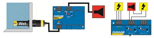
To do this, connect the hot lead of the alarm to the NC side of the relay terminal of the controller. If power is lost, the relay will be de-energized, and the alarm will sound (if there is still power to the alarm circuit itself).
