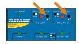
**Note:** The delay has stops on each end of its 270° rotation.
