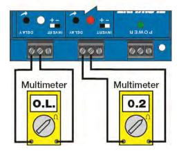
The relay contacts are true dry contacts with no voltage sourced within the relay contacts. To test, connect a Multimeter set to read Ohms.
