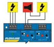
**Note:** The sensor is normally dry. In this condition, we want the relay to be energized so the alarm does not sound: i.e., the Red relay LED should be on whenever the Input LED is Amber. So we turn Invert On. If liquid comes into contact with the switch, the switch activates, the relay de-energizes, and the alarm sounds.
