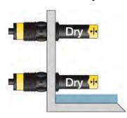
In this state, the relay will never switch, regardless if this is an Auto Fill or Auto Empty application. In this state, the relay will typically energize for an Auto Empty application and will typically deenergize for an Auto Fill application. In this state, the relay will typically energize for an Auto Fill application and will typically de-energize for an Auto Empty application.
