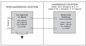
Control drawing for the LD20 Series DeltraRange level transmitters Rev. 4-24-02 approved under the entity concept as an I.S. apparatus Control Drawing: LD20CD
