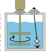
install the LD10 and LD20 series inside a still well/drop tube. The still well/drop pipe will minimize the effects created by the mixer.
