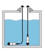
the lowest reading of liquid will be 1 foot from the bottom.
