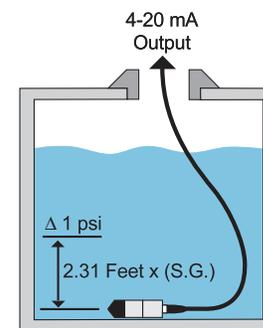
For liquids with a different SG, simply multiply 2.31 by the new SG to determine the new ratio. For example, the LD10-S041 is installed in a liquid with a SG = 0.85. The new ratio is as follows:
