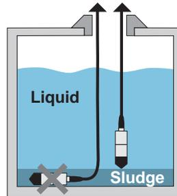
The LD10 series is designed to operate while submerged in the actual application liquid. Avoid installing the level transmitter along the bottom of the tank as materials such as sludge will build up and coat/cover the transmitter. This also includes any debris that will settle along the bottom of the tank. In these applications, it is best to suspend the transmitter above the highest level of sludge/debris that will occur.
