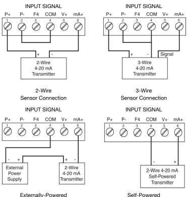
Self-Powered 2-Wire Sensor Connection
