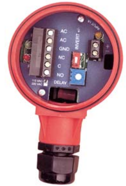
Compact Relay Controller (inside shown)
