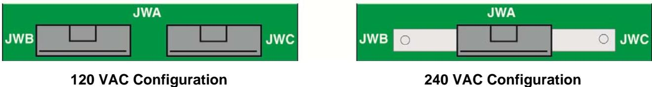
**3. Connect switched device to the relay (Relay Input Wiring):**
